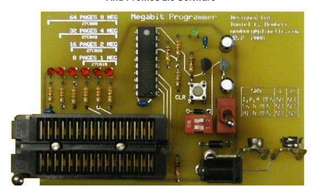
Now you can program high capacity EPROMs with the Promenade C1 or Megabit C1 Clone programmers using Promos 2.0 software. The Megabit Programmer will program the following EPROMs:
